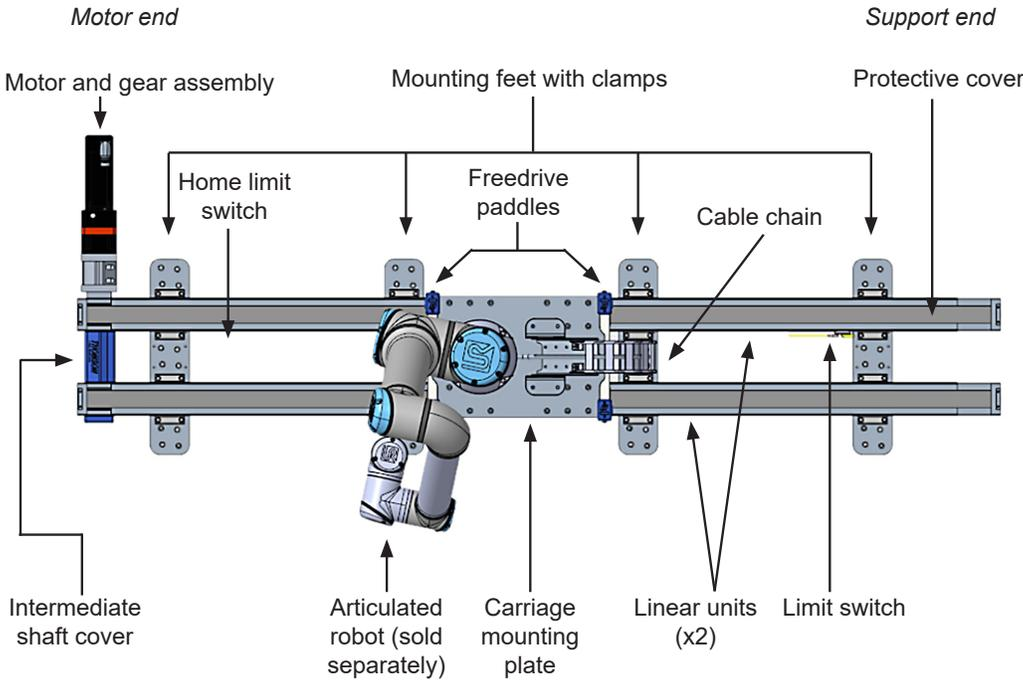
Included: Dual linear units, Kollmorgen servo motor, precision gearhead, carriage mounting plate for robot, Freedrive paddles, end-of-stroke limit switches, cable management, control box and software with 7th axis collision detection. For Universal Robots, a URcap is available for programming directly on the UR Teach Pendant.
