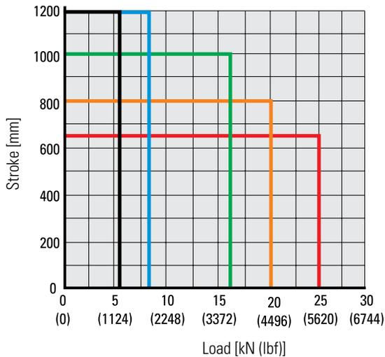
Static Compression Load vs. Stroke <sup>(2)</sup>
