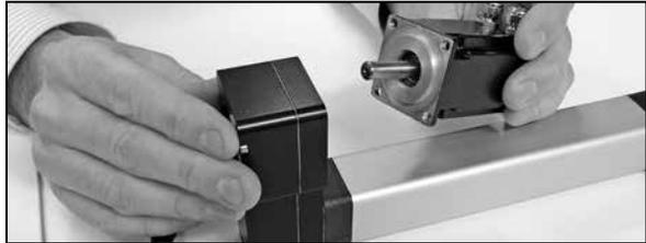
3. Use a hexagon key to tighten the coupling around the motor shaft. Correct tightening torque for PC25 models = 0.85 Nm and for PC32 and PC40 = 2.0 Nm.
