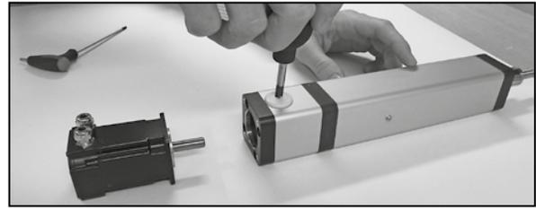
2. Press the motor shaft on to the coupling inside of the flange.
