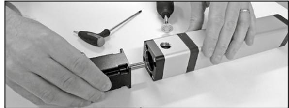
3. Bolt the motor to the flange using four screws. Tighten the screws according to table T6.3.1.
