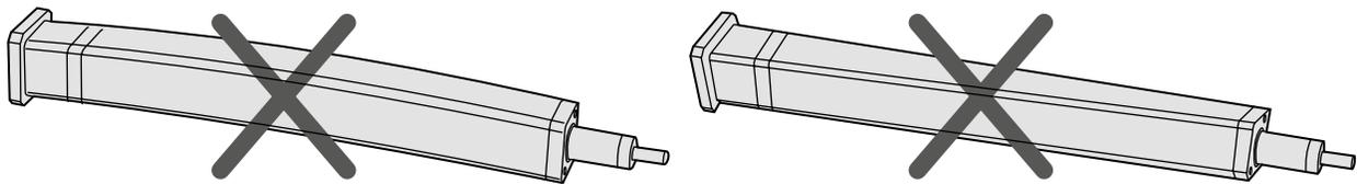
Mount actuator so that the the maximum permissible load and load torques for the input shaft or the extension tube never are exceeded during stand still or operation. See table T6.1.1 for load and load torque data for each model.
