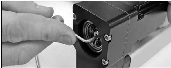
4. Bolt the motor to the flange using four screws. Tighten the screws according to table T6.3.1.
