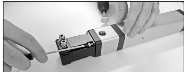
4. Use a hexagon key to tighten the coupling around the motor shaft. Correct tightening torque for PC25 models = 0.85 Nm and for PC32 and PC40 = 2.0 Nm.
