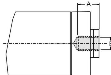
The extension tube can handle some side load (see table T6.1.1 for load and load torque data for each model) but in order to improve overall performance and life it is good practice to follow the below points even if the side loads do not exceed the maximum permitted levels.
