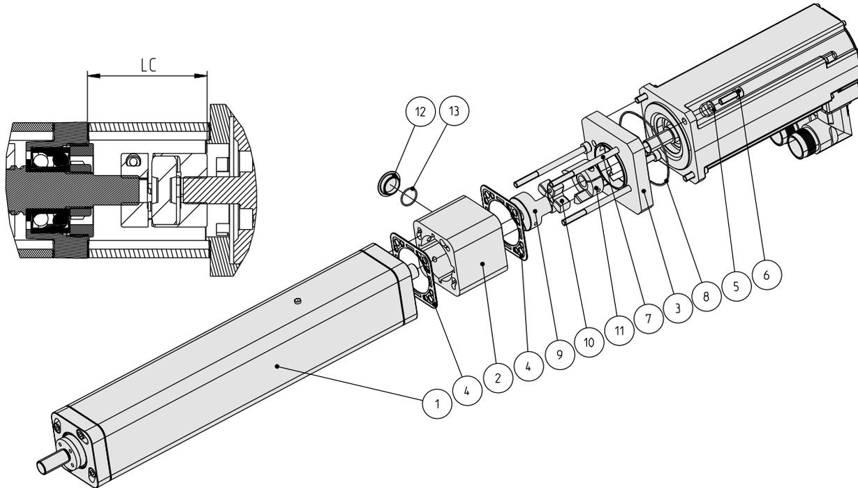
1. Remove cover lid (12) and loosen screws on the coupling half (11) closest to the motor and remove it.
