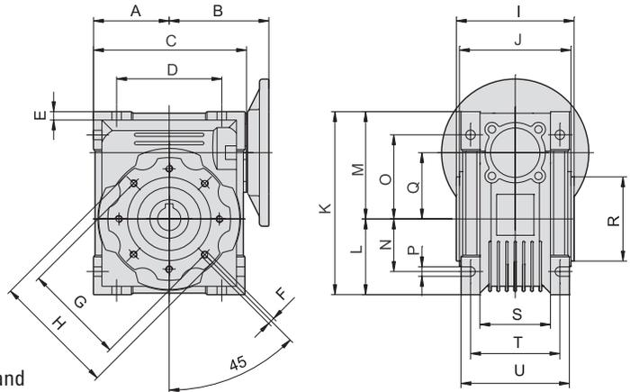
The worm gear is installed to the unit using a unit type and gear-size-specific adapter flange. No intermediate coupling is needed. The gear mounts directly to the motor and no coupling, bell house or adaptor flange is required. An optional rear clevis can be mounted to the gear by using a rear clevis adaptor flange. This can be ordered as a package either unmounted or mounted to the unit, or as separate items.
