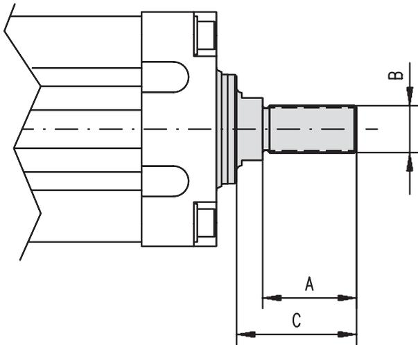
The outside thread option comes mounted from factory if this is stated in the ordering key at order. Possible types for the different unit sizes depend on the ball screw diameter of the unit, see "Ball screw diameter" in the table.
