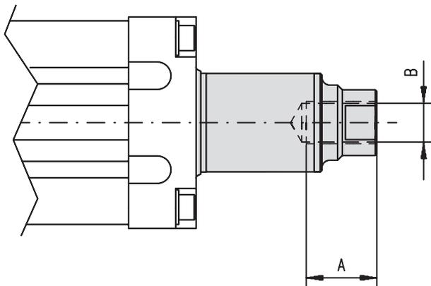
The inside thread option comes mounted from factory if this is stated in the ordering key at order. Possible types for the different unit sizes depend on the ball screw diameter of the unit, see "Ball screw diameter" in the table.
