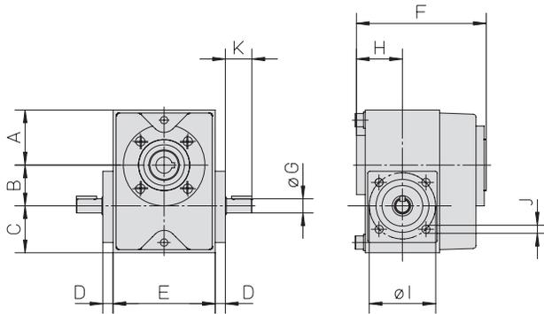
The worm gear is installed directly to the unit and requires no intermediate coupling between the two. To install the gear to the motor, a bell house flange must be used between the gear and the motor. The bell house flange, which includes a matching coupling, is ordered separately. A shaft cover can be ordered to cover the second primary shaft on the gear in case it is not being used.
