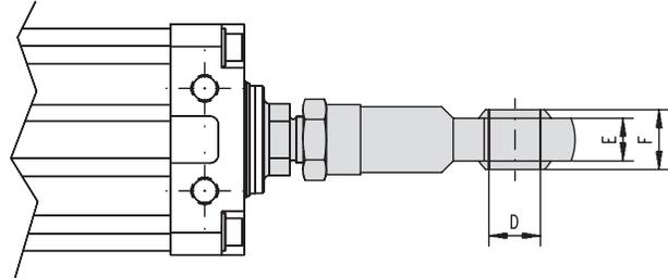
The spherical joint option can be mounted on the unit from the factory if this is stated in the ordering key at order, or can be ordered separately using the part number(s). When ordered separately, all necessary components to attach the spherical joints to the unit are included. Type M joints include a grease nipple. Note: When ordering a spherical joint separately, make sure that the extension tube end has an outside thread adapter to be able to mount it.
