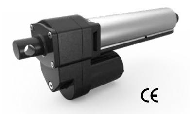
The K4x model provides the highest load rating in its class. This model incorporates all of the base K2 features with a ball screw for a 4,000 lb. (17760 N) load capability within a compact package size. The K4x includes a bi-directional wrap spring brake for load holding capability. These units are well suited for the most demanding applications where an alternative to hydraulic or air cylinders is needed or where hydraulic power sources are not available.
