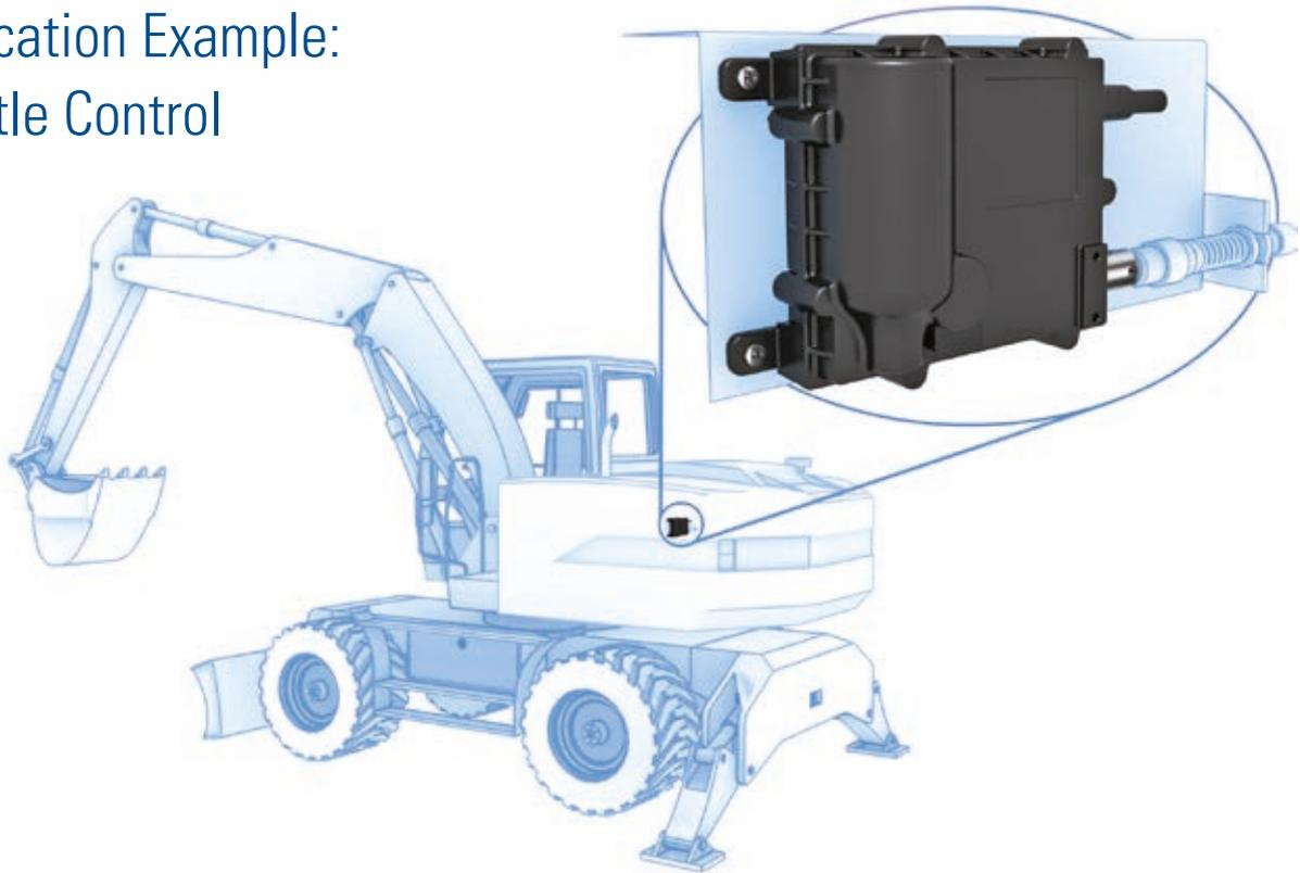
Throttle actuators allow automatic control of engine speed for reduced noise and emissions, and improved fuel economy.
