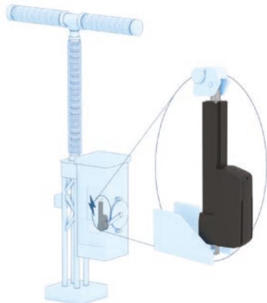
Electrical switch gears are often placed in remote locations. It is critical that power switching is executed and confirmed without fail and electric linear actuators are ideal for this task.
