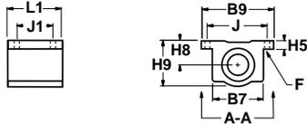
FluoroNyliner Linear Guide Twin Pillow Block Dimensions
