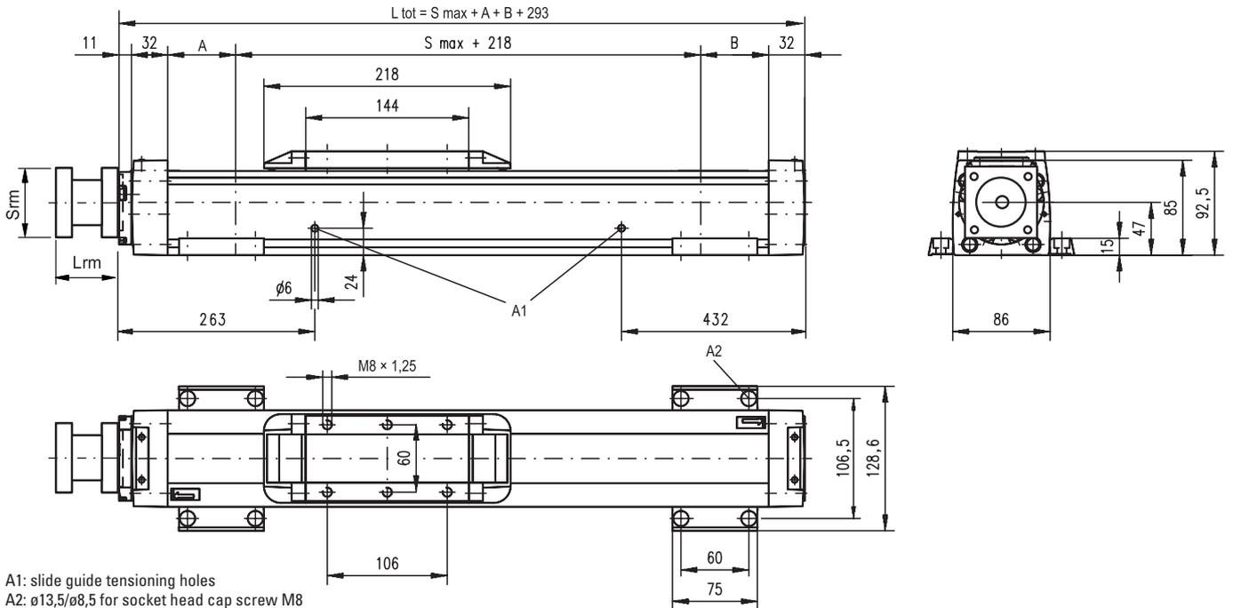
A1: slide guide tensioning holes
