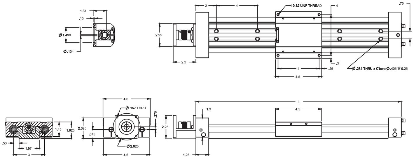
Standard NEMA23 motor dimensions are shown. Other mounting sizes are available and easily configured. Please see [www.LinearMotioneering.com](http://www.LinearMotioneering.com) for details.
