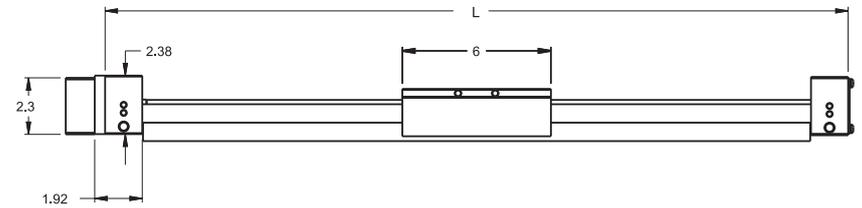
Standard NEMA23 motor dimensions are shown. Other mounting sizes are available and easily configured. Please see [www.LinearMotioneering.com](http://www.LinearMotioneering.com) for details.
