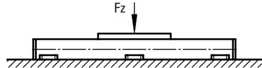
The unit must be continuously supported by a machined surface under its entire length.
