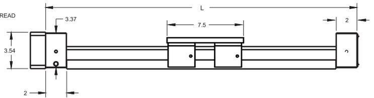
Standard NEMA23 motor dimensions are shown. Other mounting sizes are available and easily configured. Please see [www.LinearMotioneering.com](http://www.LinearMotioneering.com) for details.
