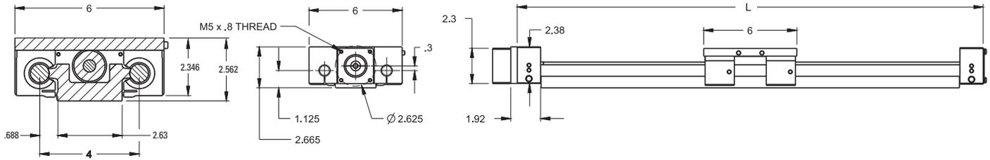
Standard NEMA23 motor dimensions are shown. Other mounting sizes are available and easily configured. Please see [www.LinearMotioneering.com](http://www.LinearMotioneering.com) for details.
