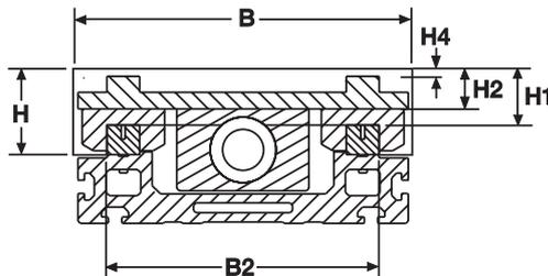
Bellows protect the unit from dirt and dust. Note that the bellows option reduces the available stroke of the unit by 28%. Bellows can be ordered and mounted at the factory - see ordering key. Bellows can also be ordered separately and fitted by the customer. In that case, order two pieces of bellows where the length of each bellows piece = stroke length of the unit  $\times$  0.86.
