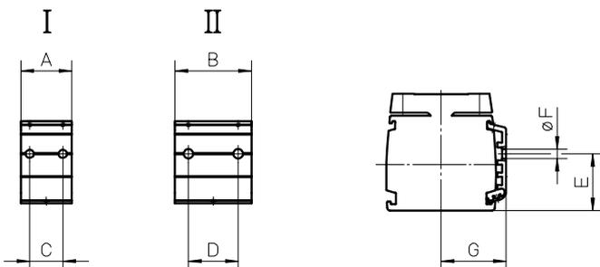
Adapter plates are fitted in the grooves along the profile and can be used to attach sensors, switches, cable ducts etc. to the unit.
