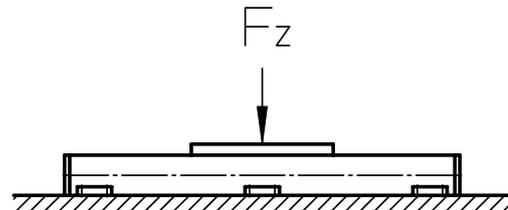
The unit must be continuously supported by a machined surface under its entire length.
