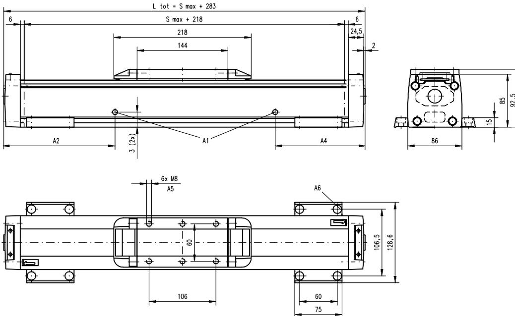
A1: slide guide tensioning holes  $\phi 6$  (MG07N), lubrication holes  $\phi 10$  (MF07N)
