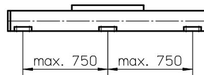
A mounting clamp must be installed at least every 750 mm to be able to operate at maximum load. Less clamps may be required if less load is being operated, see the additional technical data for more information.
