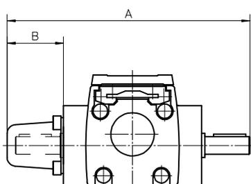
The shaft protection cover is used to cover shafts which are not being used. The covers are fitted by the customer.
