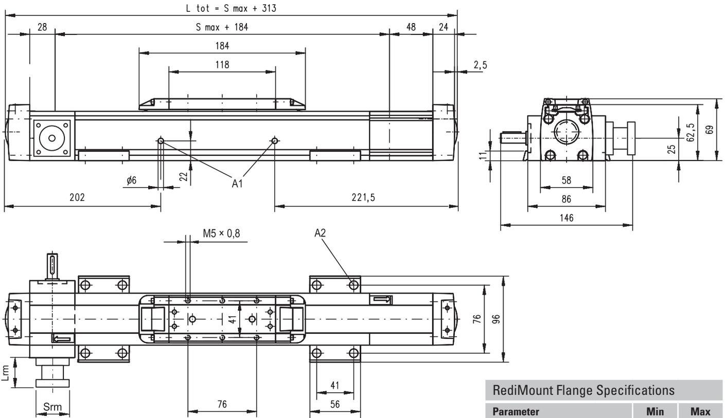
A1: slide guide tensioning holes
