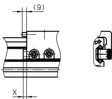
The felt pad wipers remove dust and dirt from the guides and are located on the carriage(s). They may increase the driving torque slightly but do not reduce the stroke of the unit. The felt pad wipers comes mounted from factory as standard on all WH and WHZ units but can also be ordered here as a spare part.
