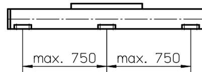
A mounting clamp must be installed at least every 750 mm to be able to operate at maximum load. Less clamps may be required if less load is being operated, see the additional technical data for more information. Units with a profile length over 4900 mm consist of two profiles where the joint between the two profiles must be adequately supported on both sides.
