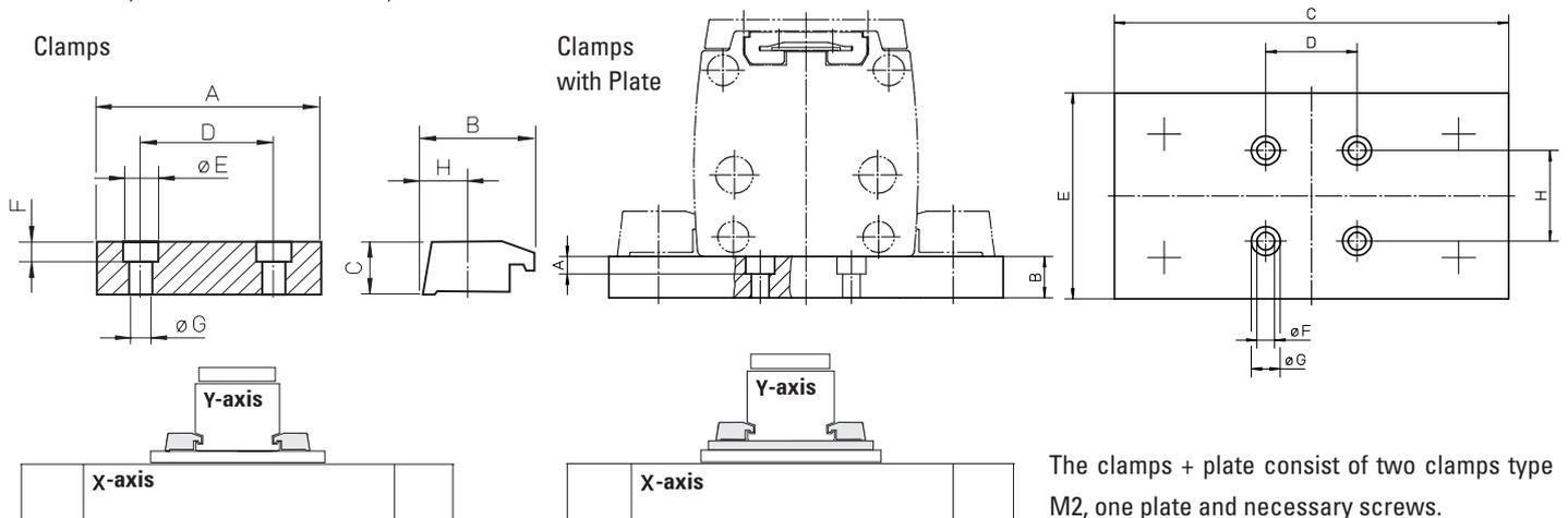
The clamps + plate consist of two clamps type M2, one plate and necessary screws.
