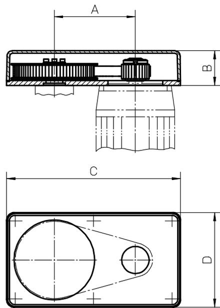
BGM belt gears can only be used on units without a RediMount flange. The belt gear comes in parts and is assembled to the unit and motor by the customer.
