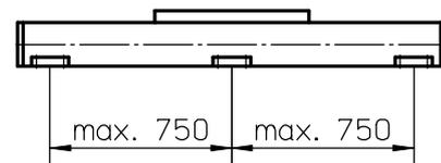
A mounting clamp must be installed at least every 750 mm to be able to operate at maximum load. Less clamps may be required if less load is being operated, see the additional technical data for more information. Units with a profile length over 6300 mm consist of two profiles where the joint between the two profiles must be adequately supported on both sides.
