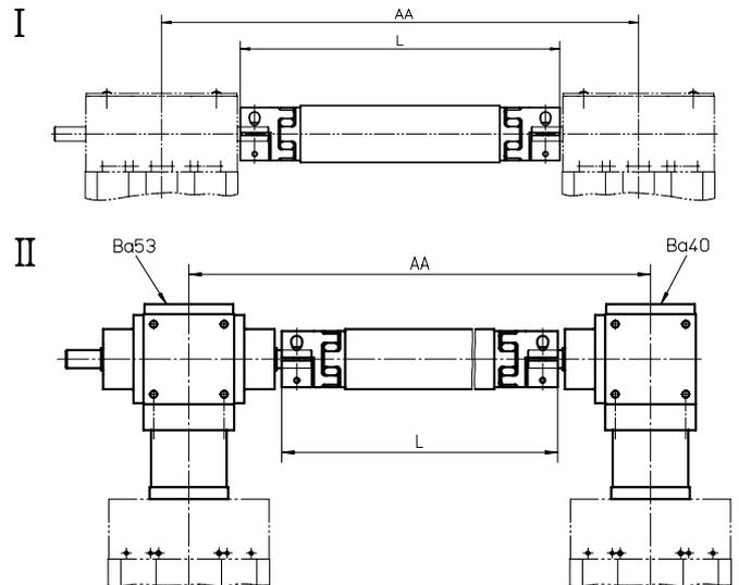
The VWZ intermediate shafts can be installed in two ways. Either directly to belt driven units (I) or to screw driven units using KRG bevel gears (II) of type VL50, VL100 or VL200. However, belt driven units with a RediMount flange can not be combined with VWZ shafts while screw driven units can, but in which case the unit must be ordered with the RediMount ID code that fits the bevel gear in question. The intermediate shaft includes tube and couplings.
