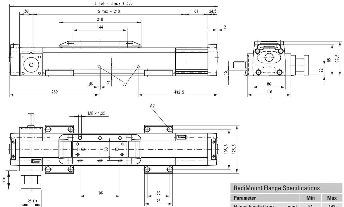
A1: slide guide tensioning holes
