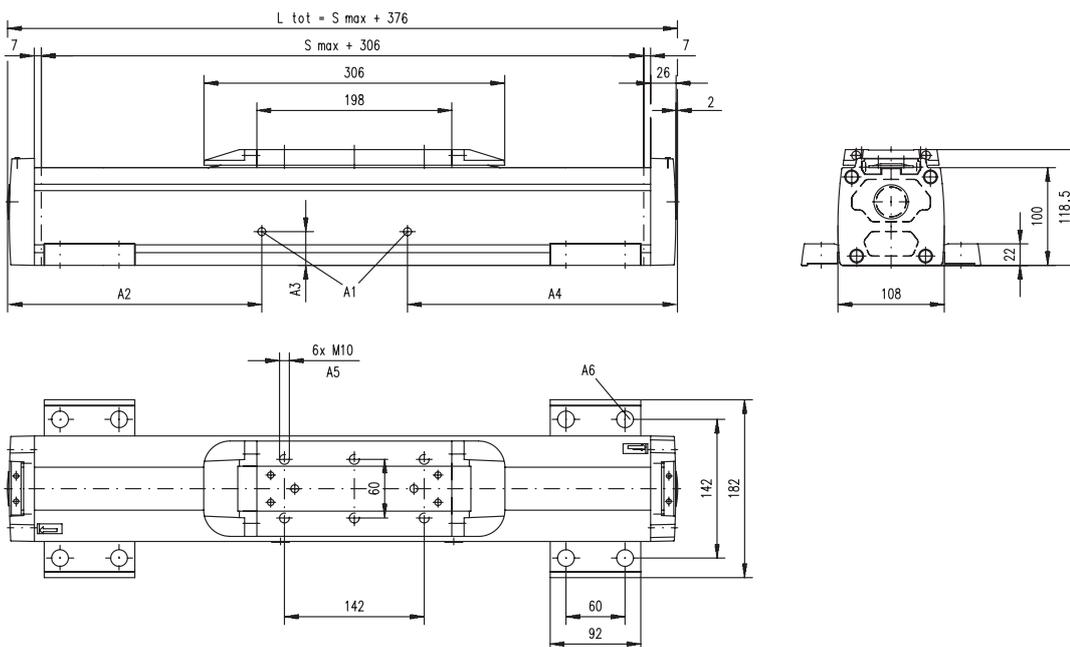
A1: slide guide tensioning holes  $\phi 6$  (MG10N),  $\phi 10$  (MF10N)
