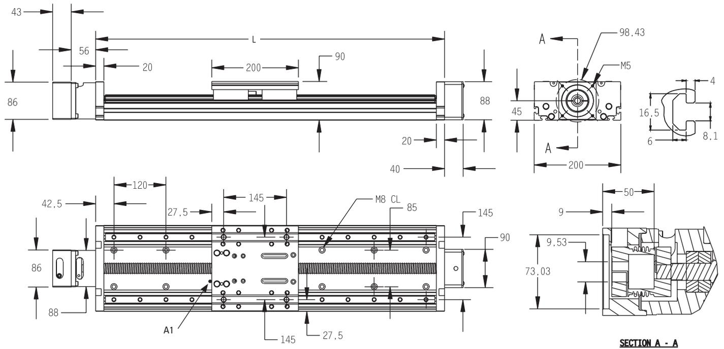
A1: lubrication nipple (using the unit with the nipple mounted makes the stroke 10 mm shorter).
