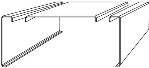
The protective shrouds are made of metal and protect the drive mechanism of the unit from dust and dirt but leave the guides unprotected. Shrouds do not reduce the stroke of the unit but they will add 4 mm to the width of the unit. Shrouds are ordered mounted from factory and are stated in the ordering key of the unit.
