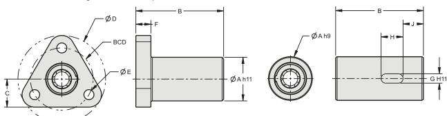
Part number example: GSC25x0500 = glide screw assembly, cylindrical nut, 0.250 inch diameter by 0.500 inch lead
