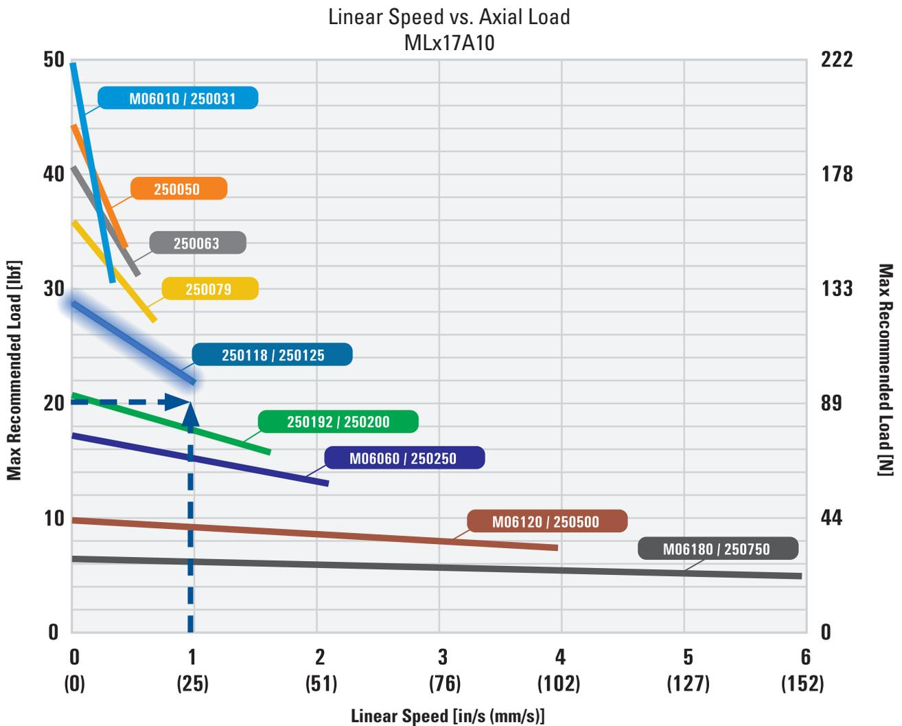
Given the force and speed requirements of 20 lbf and 1 in/s, respectively, the ideal screw is a 250118 or 250125 with this motor.
