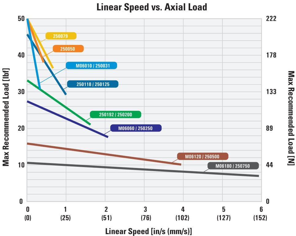
Note: Simplified performance diagrams are theoretical only and assume ideal conditions with a 24 VDC power supply, standard material lead nut and a moderate length, non-lubricated lead screw. Higher loads and speeds can be achieved. For more detailed performance plots and sizing tools, please visit [www.thomsonlinear.com/en/products/motorized-lead-screws](http://www.thomsonlinear.com/en/products/motorized-lead-screws).
