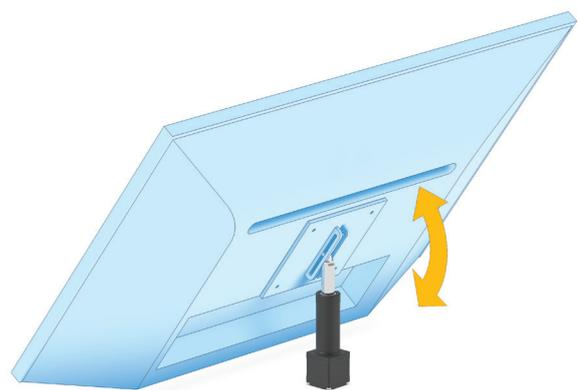
Angle adjustment is made simple when the MLA configuration is applied in monitor and plate tilting applications.
