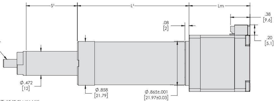
1. Molex 53253-0670 connector shown. Wire harness with Molex 51065-06000 mating connector and flying leads included with motor. For wiring diagram and connector details, see page 45.
