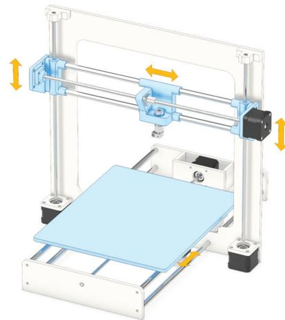
Utilizing a stepper motor linear actuator on a 3D printer can eliminate the need for couplings, bearings and supports while increasing stroke length and print volume.
