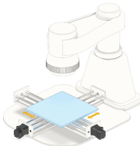
Stepper motor linear actuators optimize XY stage designs with their compactness and power.
