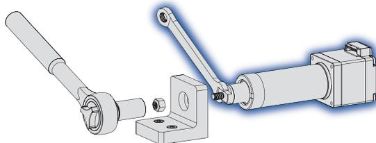
When installing your load to the end mount of an MLA assembly, always use the dedicated flats to prevent over-torquing and damaging the actuator's internal components.
