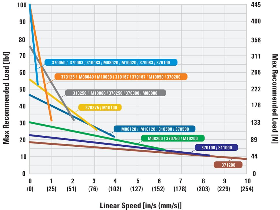
Note: Simplified performance diagrams are theoretical only and assume ideal conditions with a 24 VDC power supply, standard material lead nut and a moderate length, non-lubricated lead screw. Higher loads and speeds can be achieved. For more detailed performance plots and sizing tools, please visit [www.thomsonlinear.com/en/products/motorized-lead-screws](http://www.thomsonlinear.com/en/products/motorized-lead-screws).
