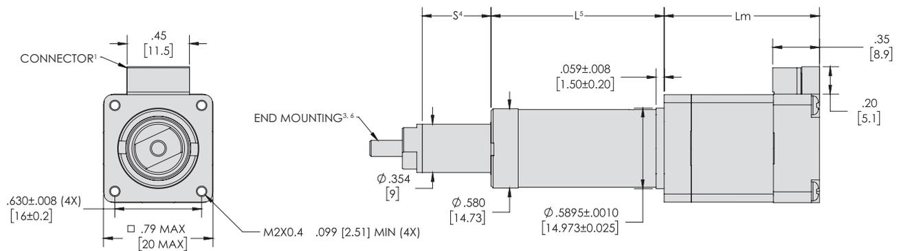
1. S6B-ZR(LF)(SN) connector shown. Wire harness with JST ZHR-6 mating connector and flying leads included with motor. For wiring diagram and connector details, see page 45.
